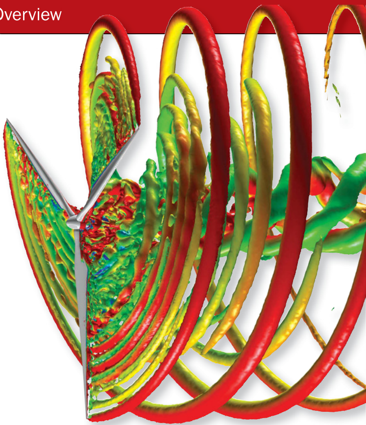
FIGURE 3: AcuSolve CFD results on a wind turbine.
