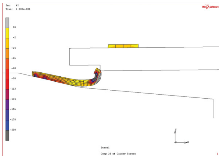
FIGURE 3: The FEA model predicts the outward rolling of the boot's heel and the subsequent loss of contact with the installation tool.
